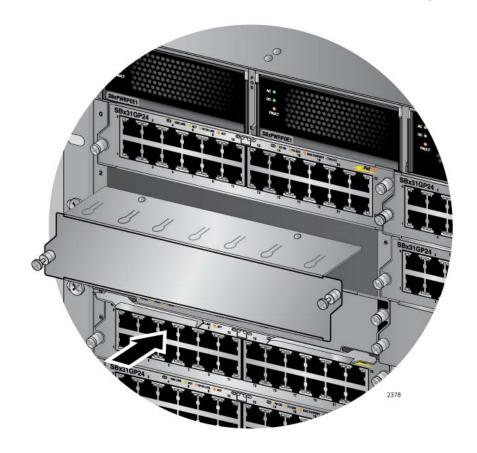
Figure 81. Installing a Blank Slot Cover
